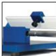
Positive tray locking connection
